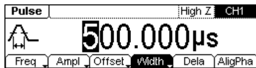
Figure 2-13 Pulse Signal Parameter Setting Interface
